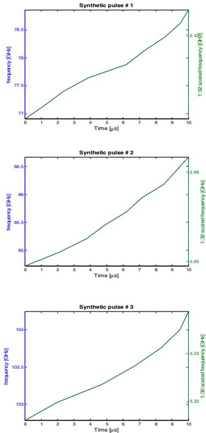
Figure 7. Nonlinear Chirp Waveforms of Matched Bands (Tank, head-on)
