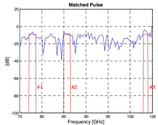
Figure 5. Bands of Matched Illumination (Tank, head-on)
