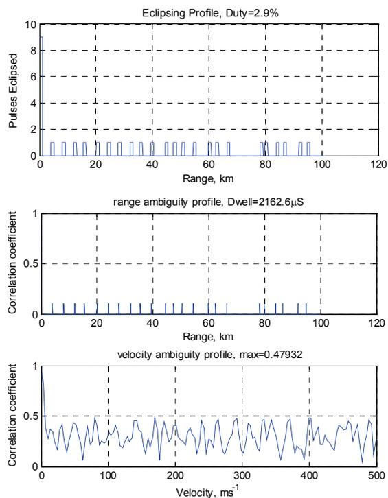
Figure 8: Results of Evolutionary Optimised Series Pulse Sequences
