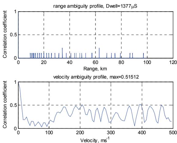
Figure 7: Results of Previous Medium PRF Pulse Sequences
