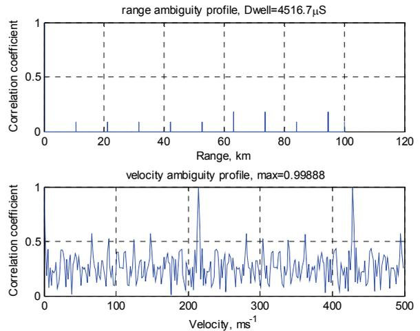
Figure 6: Results of Costas Coded Series Pulse Sequences
