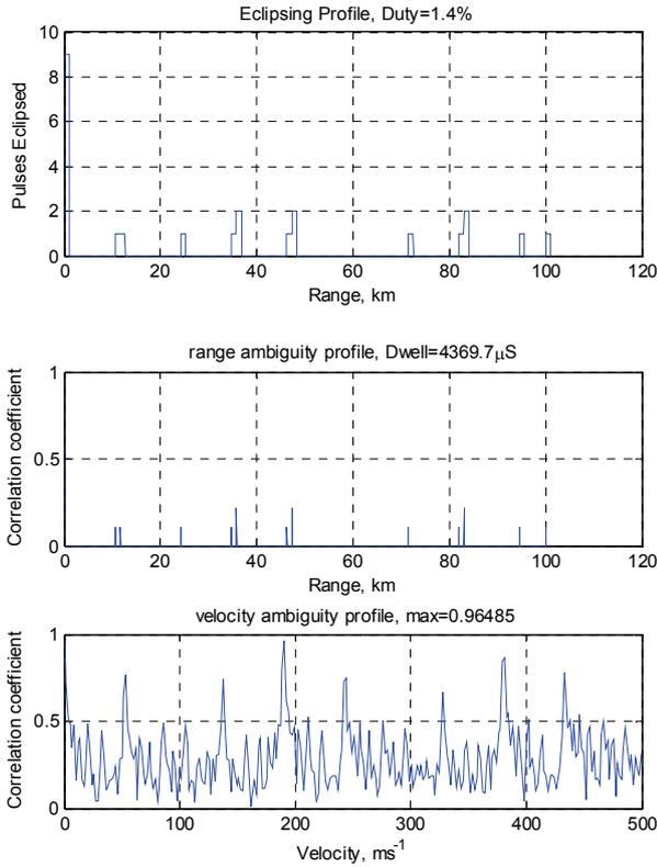
Figure 4: Results of Fibonacci Series Pulse Sequences
