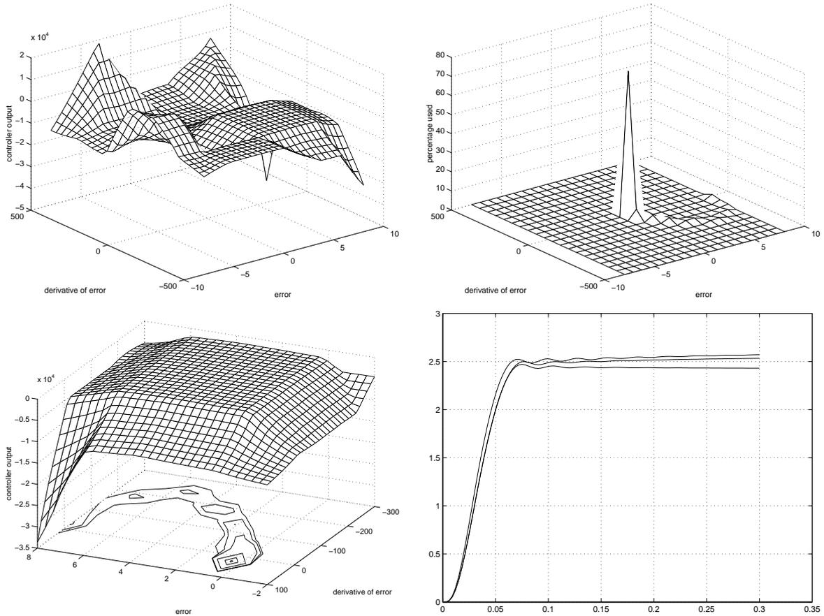
Figure 9: a)FLC surface b)usage surface c)FLC used area d)sideslip velocity
