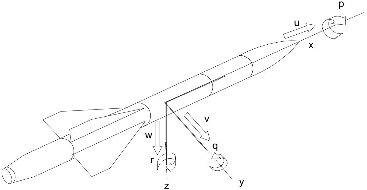
Figure 2: Airframe axes
