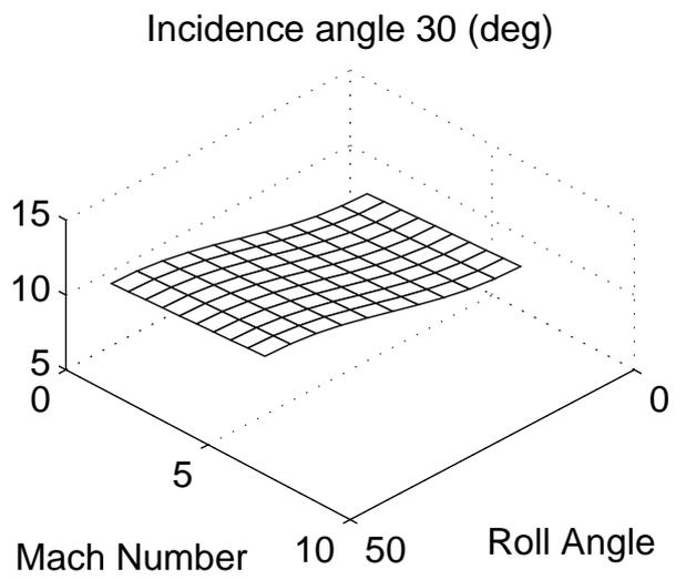
Figure 4: Centre of Pressure for different Incidence Angles
