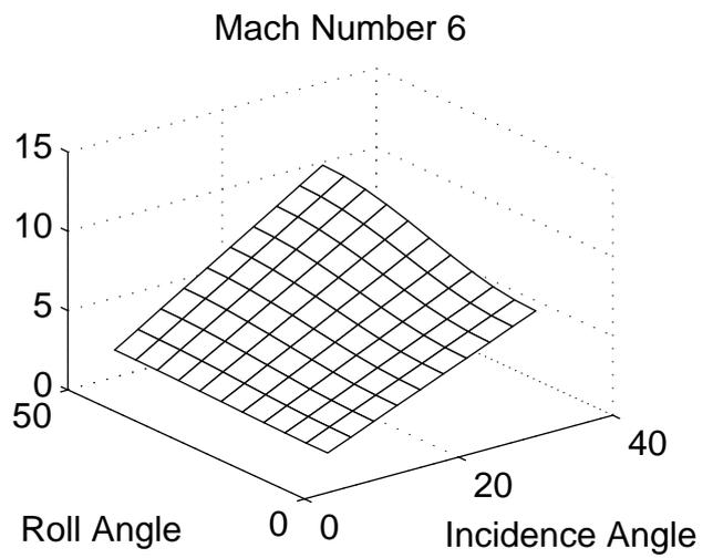
Figure 3: Centre of Pressure for different Mach Numbers
