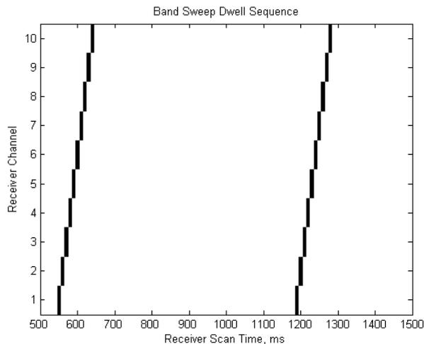
Figure 3. Fragment of band sweep reference dwell sequence for the 10 frequencies used by emitters in the test EPL. 100 dwell periods are shown, each of 10ms, giving a total 1 second section of the observation period.
