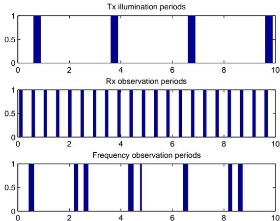
Figure 1. Example window functions for a surveillance radar rotating at 20rpm (upper plot) against an ES system with a scan antenna rotating at 120rpm (middle plot) and a non-periodic receiver dwell schedule for the one frequency channel corresponding to the emitter transmissions (lower plot). The x-axis represents a 10 second observation time and the y-axis represents whether a detection is possible at a given time or not.
