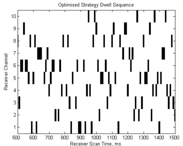
Figure 4. Fragment of an optimised dwell sequence for the 10 frequencies used by emitters in the test EPL. 100 dwell periods are shown, each of 10ms, giving a total 1 second section of the observation period.
