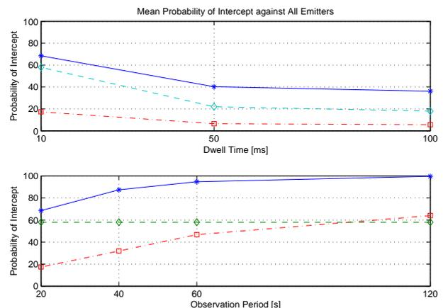
Figure 5. Overall  $P_I$  Against All Test Emitters. These two plots illustrate the mean  $P_I$  achieved against all the emitters in the test EPL by the GA-optimised strategies (solid ‘\*’) compared to the reference band sweep (dot-dash ‘□’) and channel sweep (dashed ‘◇’) sequences.
