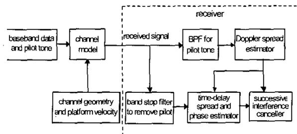
Fig. 1 Schematic block diagram of the communication system
