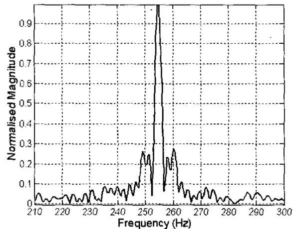
Fig. 3. Spectrum showing the three Doppler shifted/spread paths with spurious peaks at an SNR=12dB.
