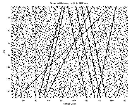
**Figure 2. Effect of Scan to Scan PRF Change**
